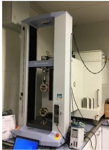
Figure 18. Single lap shear testing setup
