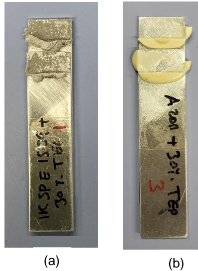
Figure 25. Fracture pattern of aluminum joints with 30% TEPs by weight: (a) 1k epoxy, (b) 2k epoxy
