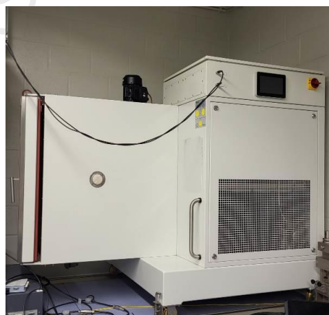
Figure 17. Climate chamber used in convection debonding tests
